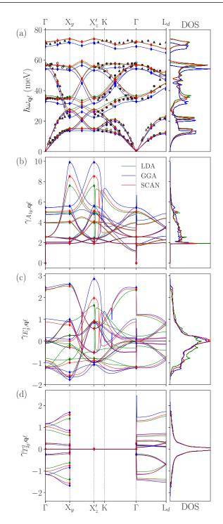
FIG. 1. The phonons and select Gruneisen parameters computed at  $\hat{\mathbf{a}}_o$  using LDA, GGA, and SCAN. Each case contains a plot along high-symmetry directions and the DOS (see Ref. [51], Table SI, for definitions of **q**). Diamonds are computed using DFT and corresponding lines are a Fourier interpolation. (a) The phonons are compared with experimental results (open markers [41] and closed markers [61]). (b–d) Generalized Gruneisen parameters.
