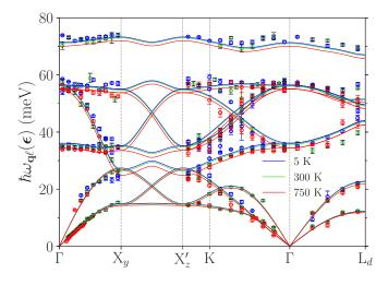
FIG. 6. The phonons computed within the QHA ( $\mathcal{N} \leq 4$ ) using SCAN (lines) and inelastic neutron scattering measurements (open circles) at T = 5, 300, 750 K along high-symmetry directions. The same color scheme is used for QHA and INS.
