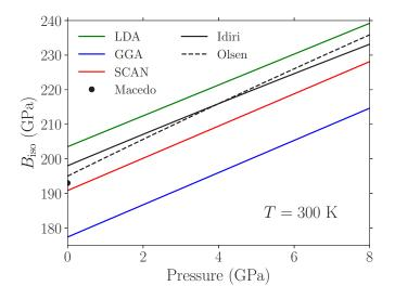
FIG. 8. The isothermal bulk modulus as a function of pressure at T = 300 K. The experimental curves were extracted from the published equations of state [82,83]; the zero-pressure result is from Ref. [42]. The theoretical results were computed using the QHA with  $\mathcal{N} \leq 4$  to leading order in pressure for LDA, GGA, and SCAN.
