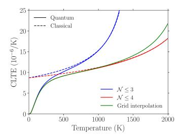
FIG. 4. The coefficient of linear thermal expansion as a function of temperature for the strain grid interpolation and Taylor series parametrizations of  $V_{qh}$  (using LDA). The classical results are shown as dotted lines.
