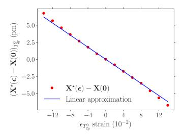
FIG. 9. The oxygen basis atom displacements projected onto the  $\Gamma$ -point  $T_{2g}^0$  vector as a function of  $\epsilon_{T_{2g}^0}$ . The circles are the result of minimizing  $\mathcal{V}_{\Gamma}$  at the specified value of strain, and the solid line is computed by the linear approximation [Eq. (B4)].
