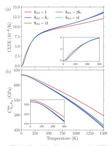
FIG. 3. (a) The coefficient of linear thermal expansion (CLTE) and (b) identity strain elastic constant  $C_{A_{1g}A_{1g}}^{iso}$  as a function of temperature for increasing supercell sizes (i.e.,  $\hat{\mathbf{S}}_{BZ}$ ) computed using QHA (LDA,  $\mathcal{N} \leq 4$ ). The insets focus on the low-temperature regime. A Fourier interpolation mesh of  $10\hat{\mathbf{l}}$  was used in all cases.
