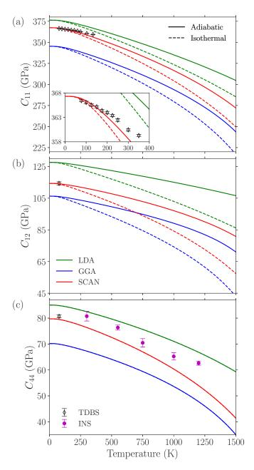
FIG. 7. The elastic constants (a)  $C_{11}$ , (b)  $C_{12}$ , and (c)  $C_{44}$  computed using QHA ( $\mathcal{N} \leq 4$ ) with LDA, GGA, and SCAN and our TDBS (diamonds) and INS (circles) measurements. Open markers and solid lines denote adiabatic conditions whereas dashed lines and solid markers denote isothermal conditions. For  $C_{44}$ , adiabatic and isothermal conditions yield the same results.
