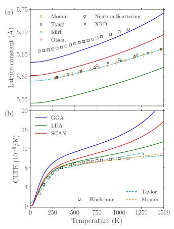
FIG. 5. The lattice parameter and coefficient of linear thermal expansion computed within QHA ( $\mathcal{N} \leq 4$ ) using LDA, GGA, and SCAN (solid lines) in addition to experimental results. (a) The lattice parameter: QHA (solid lines), our XRD (black x) and neutron scattering measurements (circle), and previous experimental results [37–39,82,83,84]. (b) The coefficient of linear thermal expansion: QHA (solid lines) and previous experimental results [37–39].
