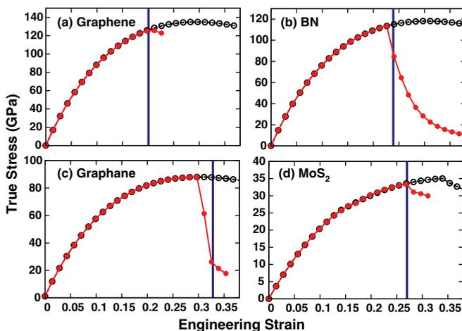
FIG. 1. (Color online) True stress  $\sigma$  vs engineering strain  $\varepsilon$  for (a) graphene, (b) BN, (c) graphane, and (d) MoS<sub>2</sub> under equibiaxial strain. Black lines and open circles are for the primitive unit cell; red lines and solid circles are for the  $K$  cell. The strain at which a phonon mode goes soft at the  $K$  point is indicated by a blue line.
