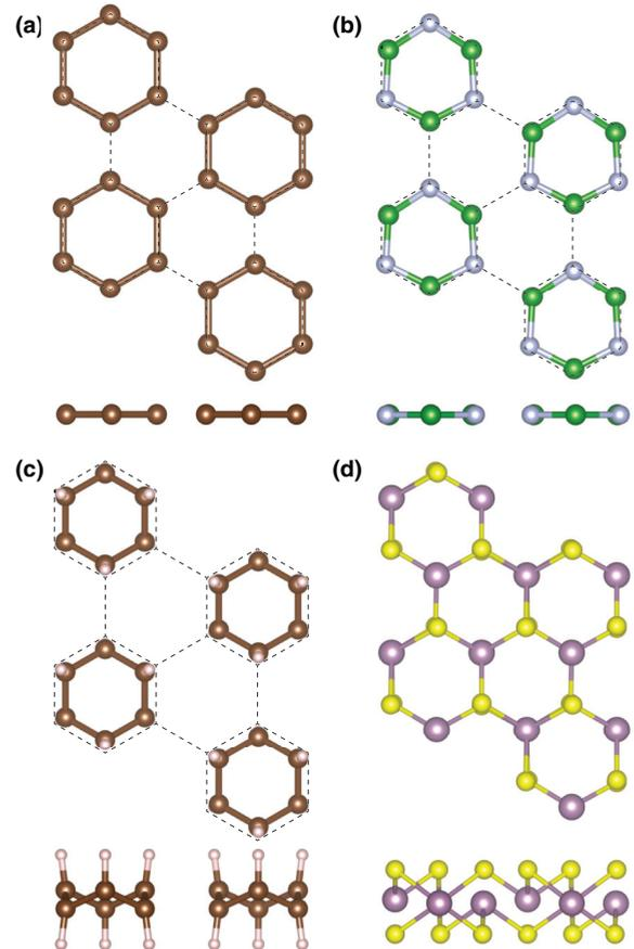
FIG. 2. (Color online) Top and side orthographic projections of the distorted structures for (a) graphene, (b) BN, (c) graphane, and (d) MoS<sub>2</sub> at equibiaxial strains of 0.212, 0.240, 0.328, and 0.270, respectively. The C, B, N, H, Mo, and S atoms are represented as brown, green, silver, white, purple, and yellow spheres, respectively. Dashed lines indicate the undistorted strained lattice.
