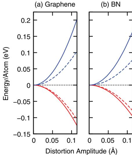
FIG. 4. (Color online) Change in electronic (red) and elastic (blue) energies as a function of soft mode distortion amplitude for the  $K$ -cell structures of (a) graphene and (b) BN at equibiaxial strains (dashed lines) of 0.212 and 0.240, respectively, compared to that at zero strain (solid lines).
